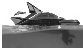
Note how far the propeller extends below the bottom of this boat.
