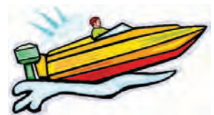
Driving with the boat trimmed like this drops the propeller deeper in the water.
